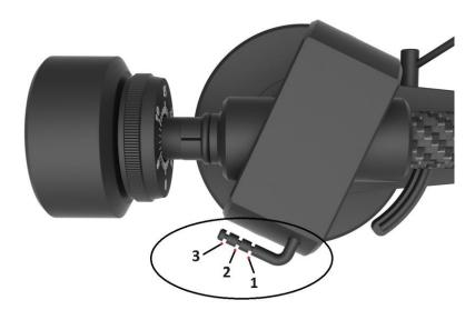
Hang the loop of the thread of the anti-skating weight in the groove of the anti-skating stub (9) corresponding to the downforce applied to your cartridge and hang the thread in the groove of the wire support (8).
